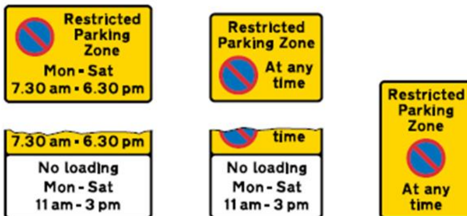
Figure 15-2 Examples of signs indicating a prohibition of waiting and loading in a restricted parking zone
